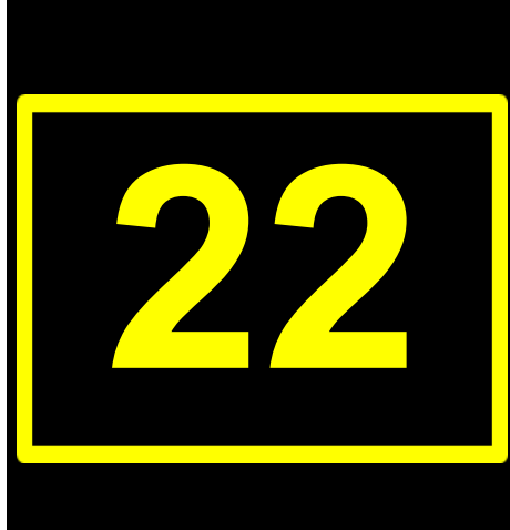
Figure 2-5 Runway Location Sign
