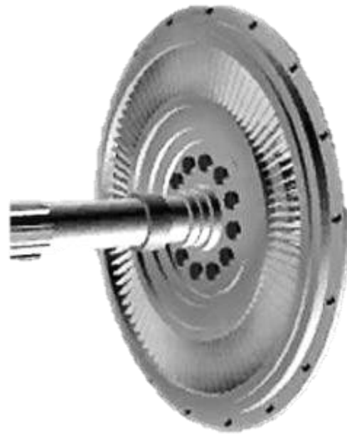
Figure 3.2-20 Turbine Rotor Blades & Stator Vanes
